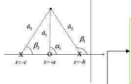
$k \frac{|s_{p} + a|}{|s_{p} + b||s_{p} + c|} = 1$   $k = \frac{|s_{p} + b||s_{p} + c|}{|s_{p} + a|} = \frac{d_{2} \cdot d_{3}}{d_{1}}$
